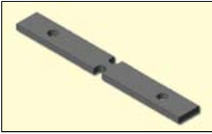
Figure 2. VRC standardized 6016-T651 aluminum notched-beam specimen (nominally 4 \times 0.5 \times 0.125 inch) fabricated in quantity to study fatigue. In use, one hole mounts beam to shaker, while other mounts standard tip mass. Intended fatigue failure area is between symmetric round-end notches.
