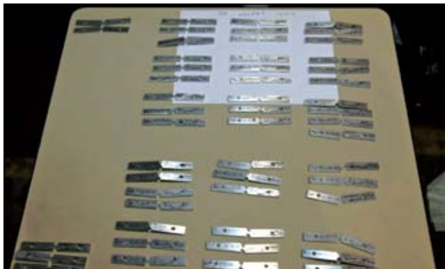
Figure 12. Fatigue specimens broken during this examination.
